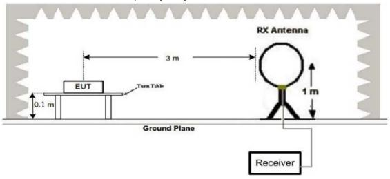
(2) Radiated Emission Test-Up Frequency 30MHz~1GHz
