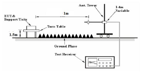
The radiated emission Below 1GHz tests were performed in the 10 meters chamber test site, above 1GHz tests were performed in the 3 meters chamber test site A, using the setup accordance with the ANSI C63.10-2013. The specification used was the FCC 15.209, and FCC 15.407 and RSS-247, RSS-Gen limits.
