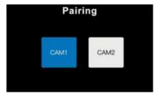
(2) Press the OK key in the selected icon to pair the video channel, and the corresponding channel icon will show the Pairing...;start the camera by long pressing the power button on the back of 2s and pair after 8 seconds.
