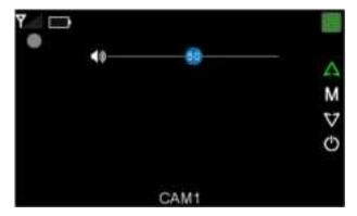
(9) If you press the OK key under the volume bar, you can mute or cancel the mute, and you can press the MENU key to directly exit the volume adjustment;
