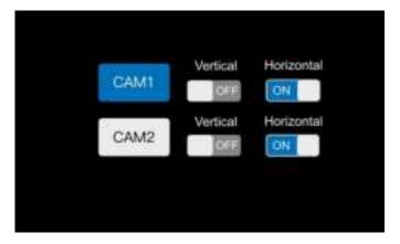
You can set the horizontal and vertical images of the camera picture; Vertical mirror: close when set to OFF, open when set to ON, the default is OFF; Horizontal mirror: close when set to OFF, open when set to ON, default to ON;
