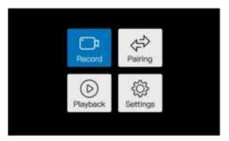
The blue highlight indicates that the icon is selected and can be selected through VOL + / VOL-movement. The main menu contains 4 ICONS, respectively: video, docking, playing and setting;
