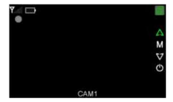
(8) Press VOL + / VOL-key under the current page, the alarm volume bar will pop up, and can adjust the alarm sound, support continuous series, the adjustment range is 0~99; press MENU key to exit directly;
