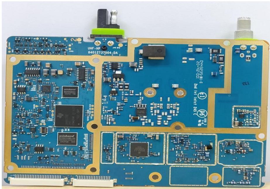
**RF board without Shields (Bottom)**
