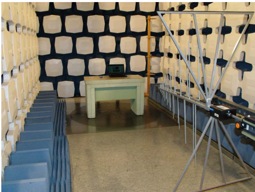
Figure 2: Radiated emission test - SAC
