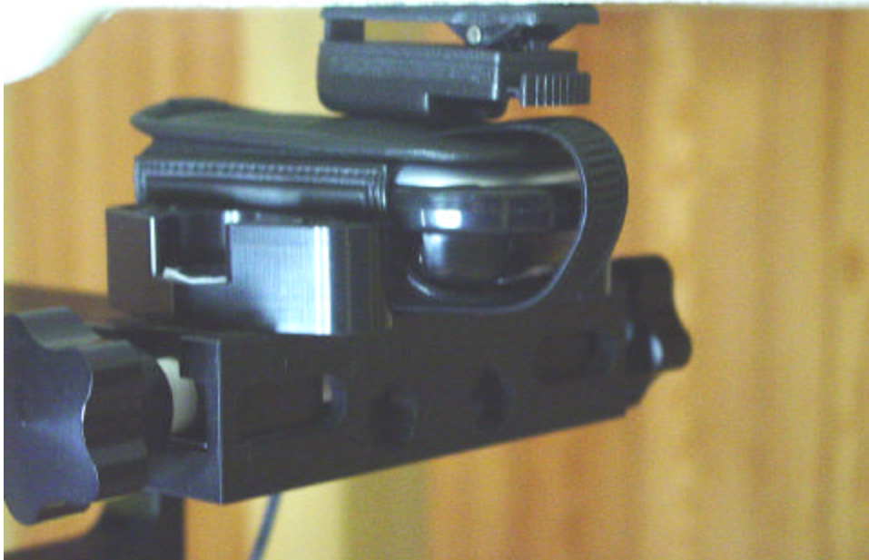
Figure 12.5 body SAR setup (with holster)
