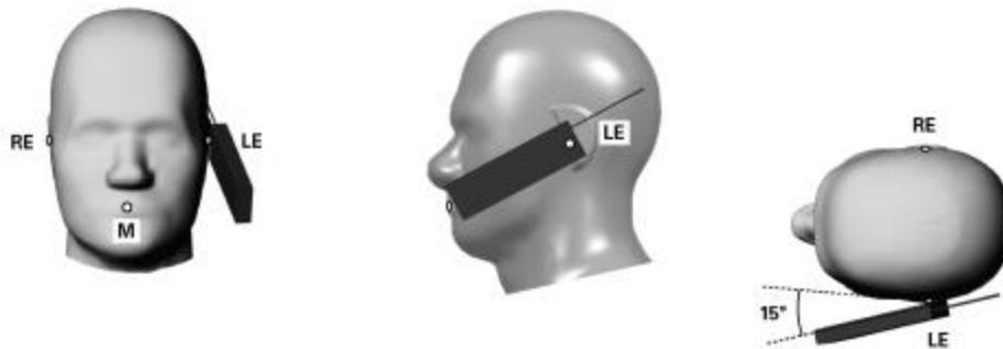
Figure 9.3 - Phone position 2, “tilted” position.
