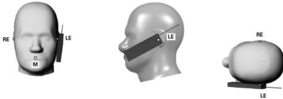
Figure 9.3 - Phone position 1, “cheek” or “touch” position.
