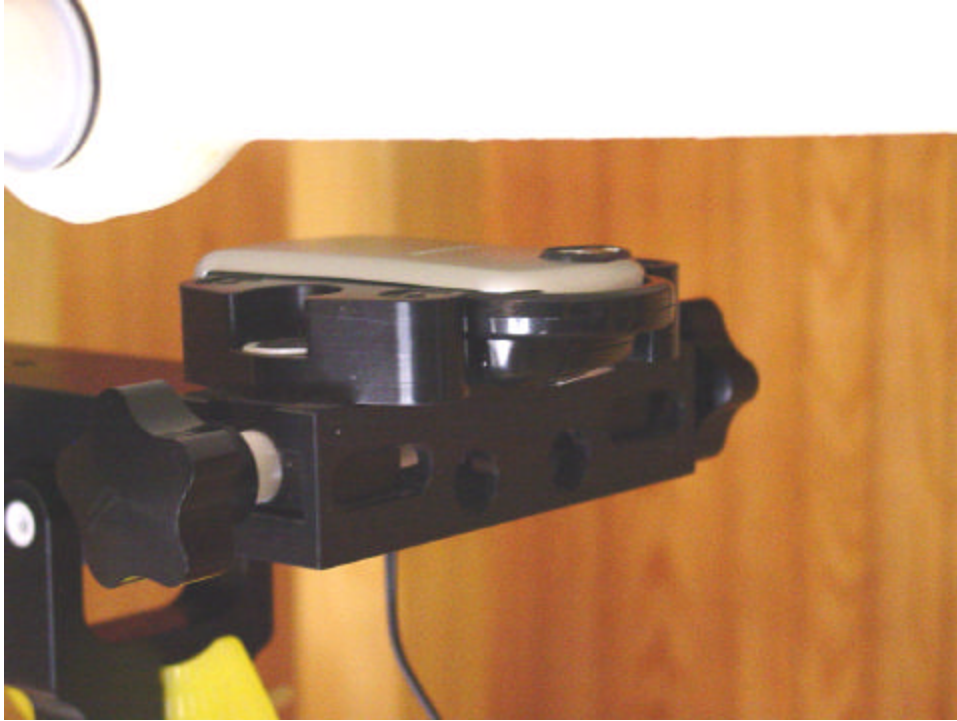
Figure 12.4 body SAR setup (with 25mm air separation)
