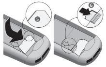
Insert battery in the phone sideways ⊘, then press downwards until it engages <sup>(3)</sup>.
