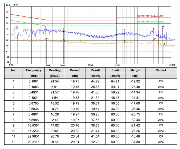
\*\*\*Note: 1).Pre-scan all modes and recorded the worst case results in this report (GFSK MCH). 2). Result = Reading + Correct, Margin = Result – Limit.
