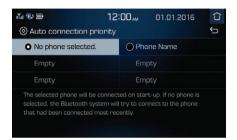
When the engine is running, the selected Bluetooth device is automatically connected. If you fail to connect the selected device, the previously-connected device is automatically connected, and if it also fails, then it tries to connect all paired devices sequentially.
