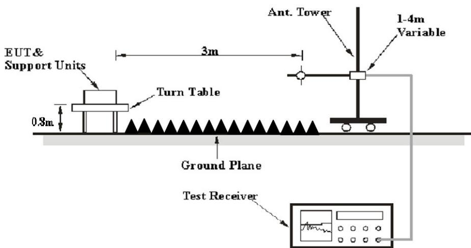
The radiated emission tests were performed in the 3 meters, using the setup accordance with the ANSI C63.4-2014. The specification used was the FCC 15.209 and FCC 15.319 (g) limits.
