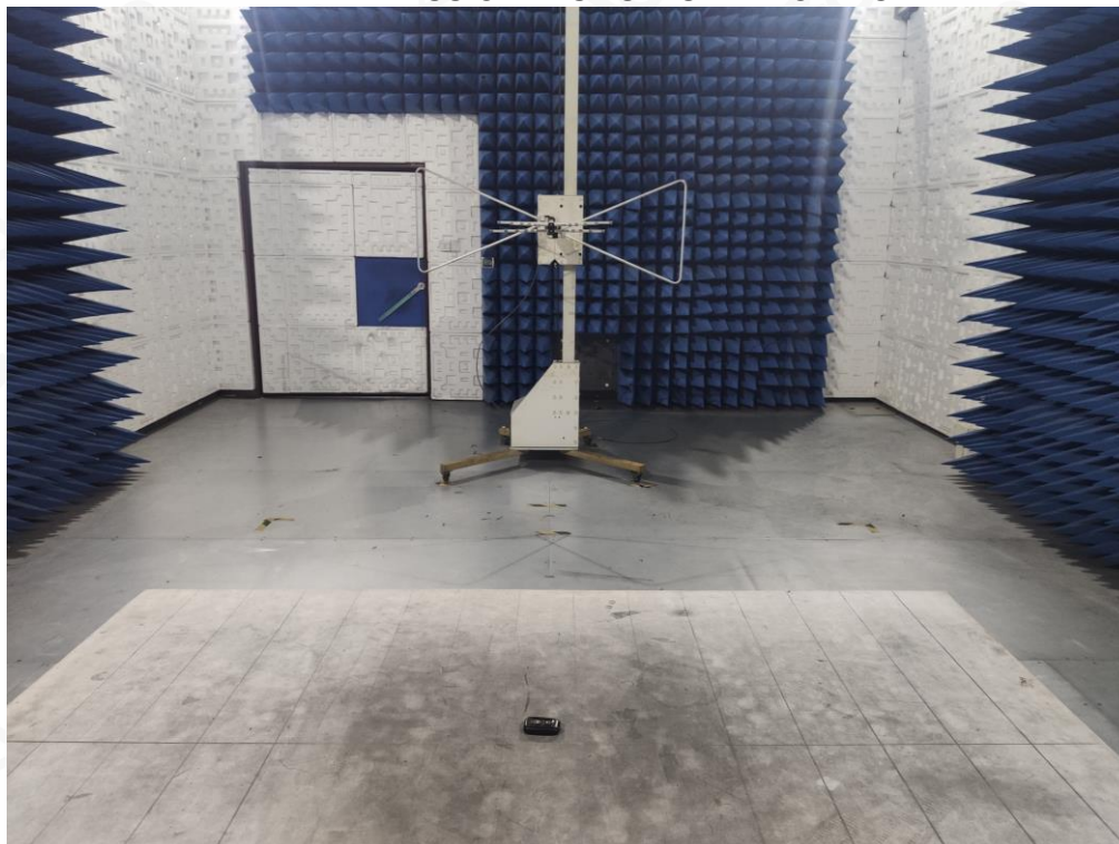
RADIATED EMISSION TEST SETUP ABOVE 1GHZ
