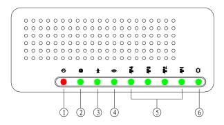
There area eight indicators on the front panel of the ZXV10 W300. These indicators indicate the service running status of the ZXV10 W300. The indicates are described in the table below.
