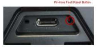
2. Gently insert a paperclip into the hole and tap the Pin-hole Fault Reset Button with light pressure.
