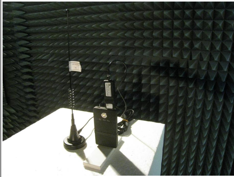
RADIATED EMISSIONS: EUT WITH RA3156.03.00.00 ANTENNA
