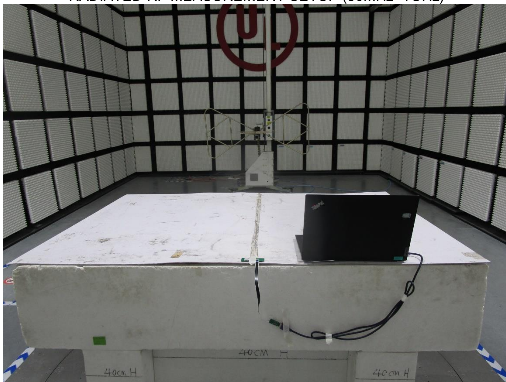
RADIATED RF MEASUREMENT SETUP (Below 30MHz)
