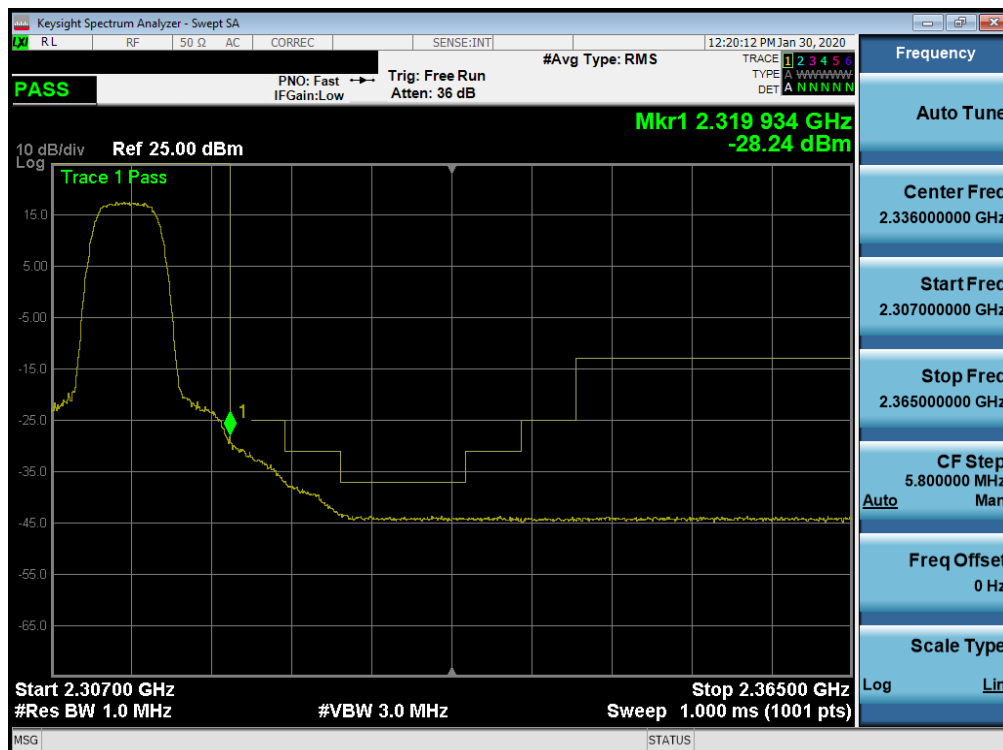
Plot 7-151. Upper Extended Band Edge Plot (Band 30 - 5.0MHz QPSK - Full RB Configuration)
