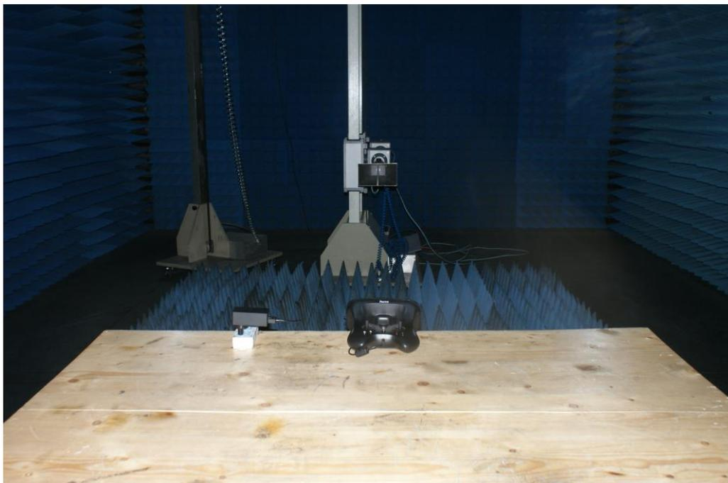
**Photograph 7: Set-up for Conducted Emission on AC Mains**
