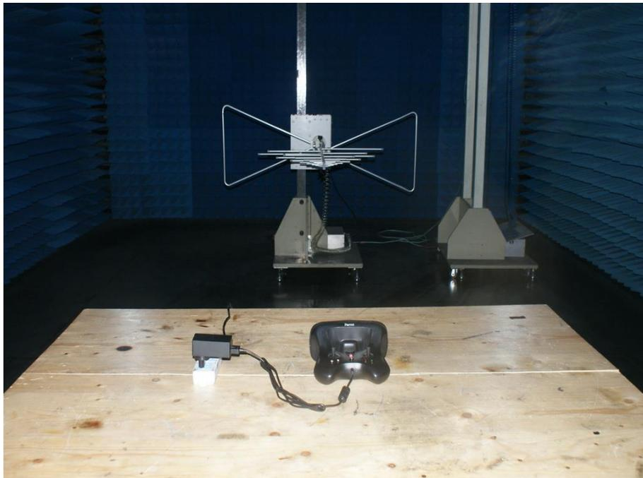
**Photograph 3: Set-up for Radiated Spurious Emission, 1GHz- 18GHz**
