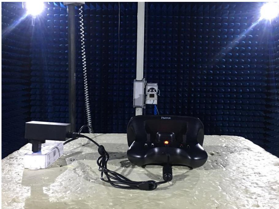
**Photograph 5: Set-up for Radiated Emission, below 1GHz**
