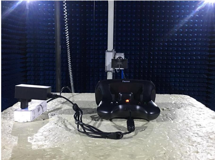
**Photograph 4: Set-up for Radiated Spurious Emission, 18GHz - 26.5GHz**
