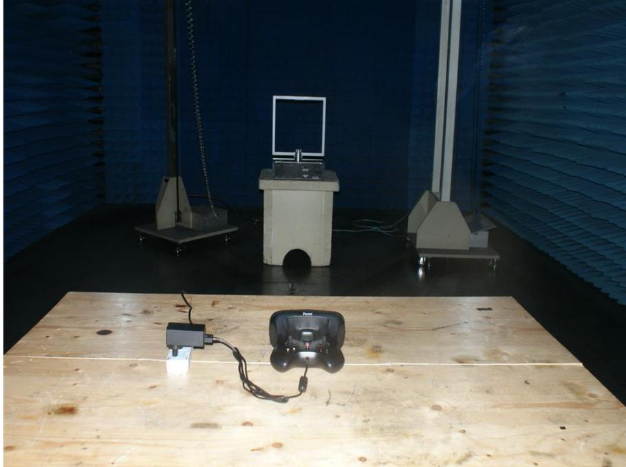
**Photograph 2: Set-up for Radiated Spurious Emission, 30MHz - 1GHz**
