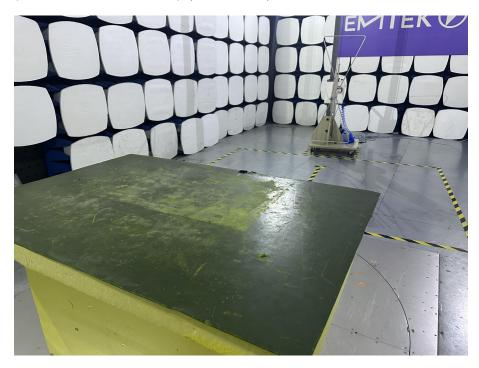
Spurious Emission Test Setup (Above 1GHz)
