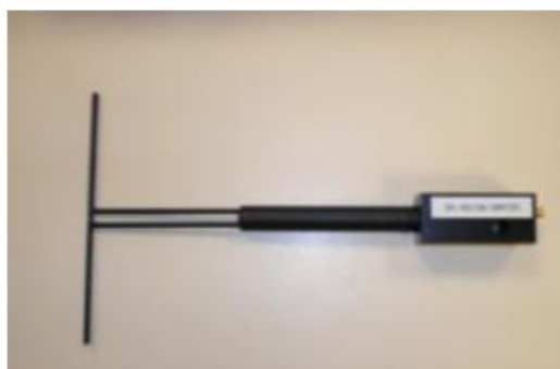
Figure 1 – Satimo COMOSAR Validation Dipole
