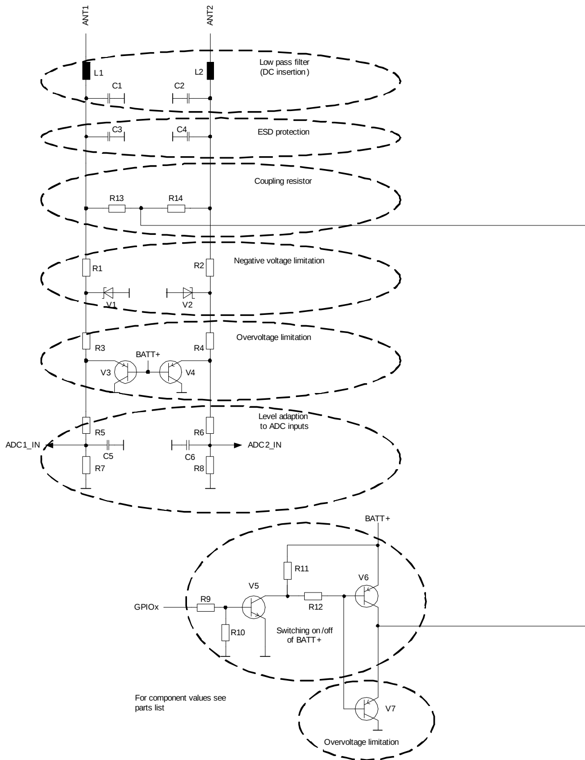
Figure 29: Antenna detection circuit sample - Schematic
