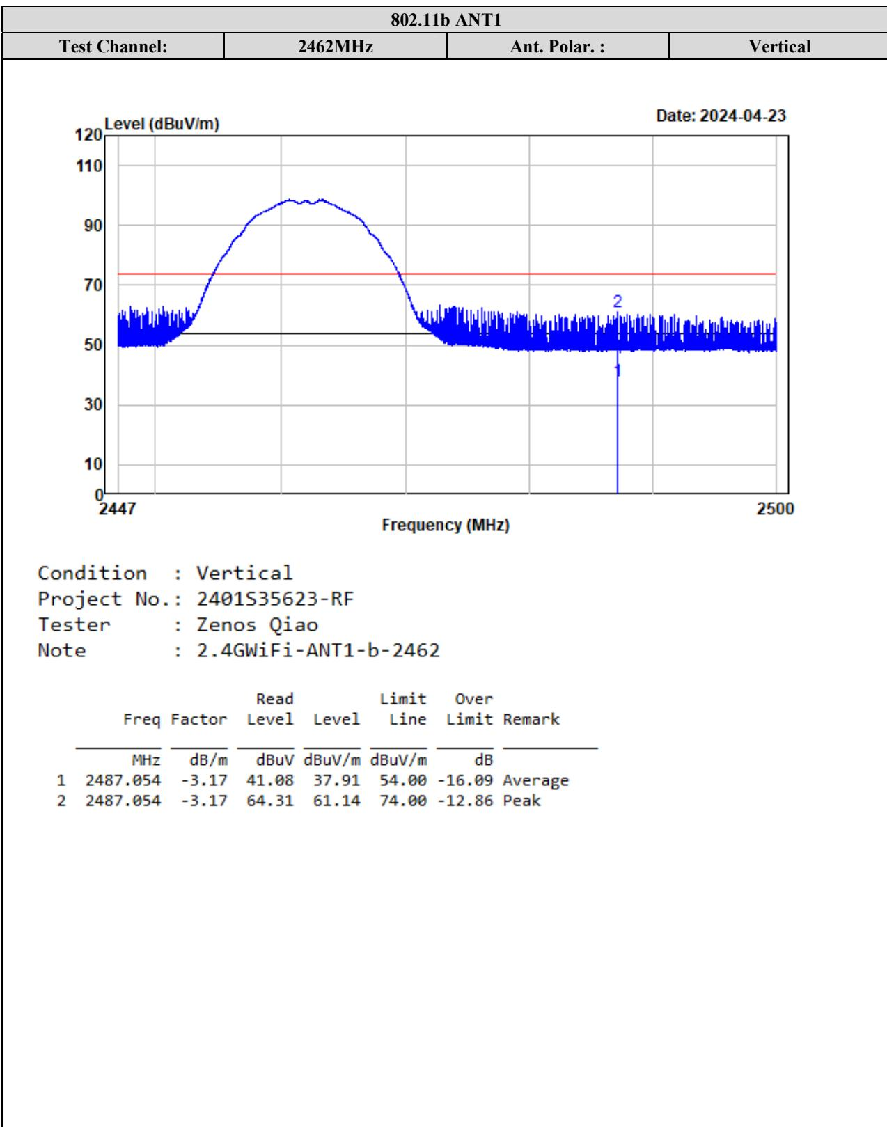
**Test plots for Harmonic Measurements (Radiated):**
