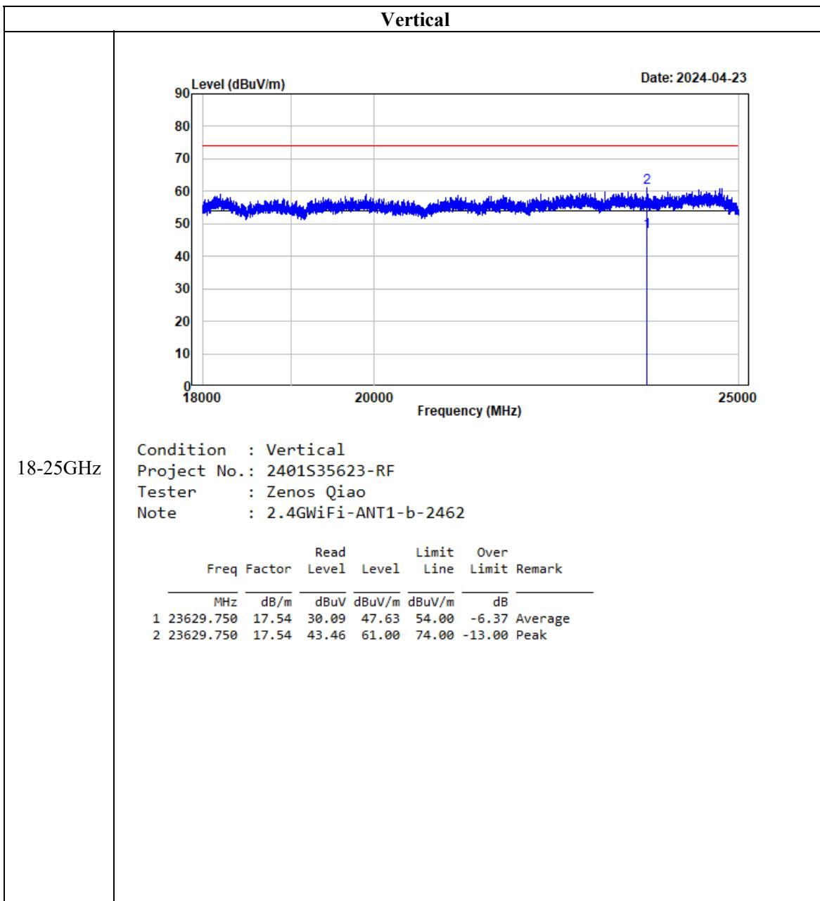
**For module YL43456****Test plots for Band Edge Measurements (Radiated):**
