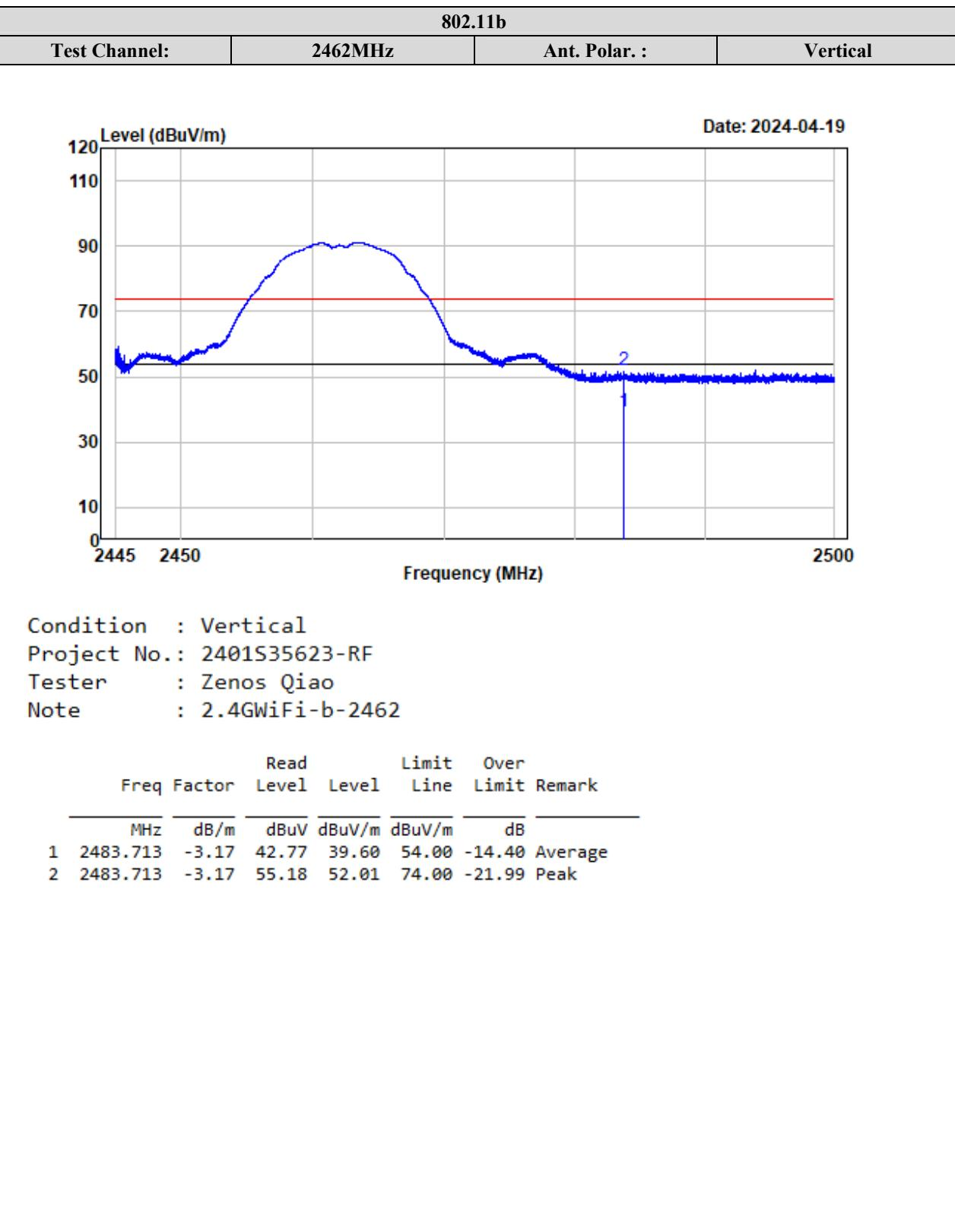
**Test plots for Harmonic Measurements (Radiated):**
