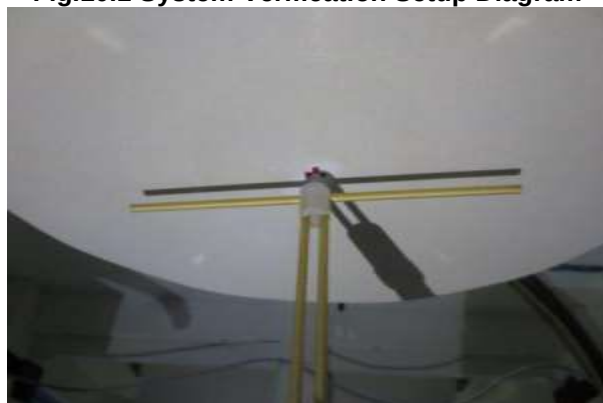
Fig.10.2 Photo of Dipole setup
