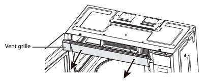
4 Replace the charcoal filter. Make sure that the wire mesh is visible from the front.
