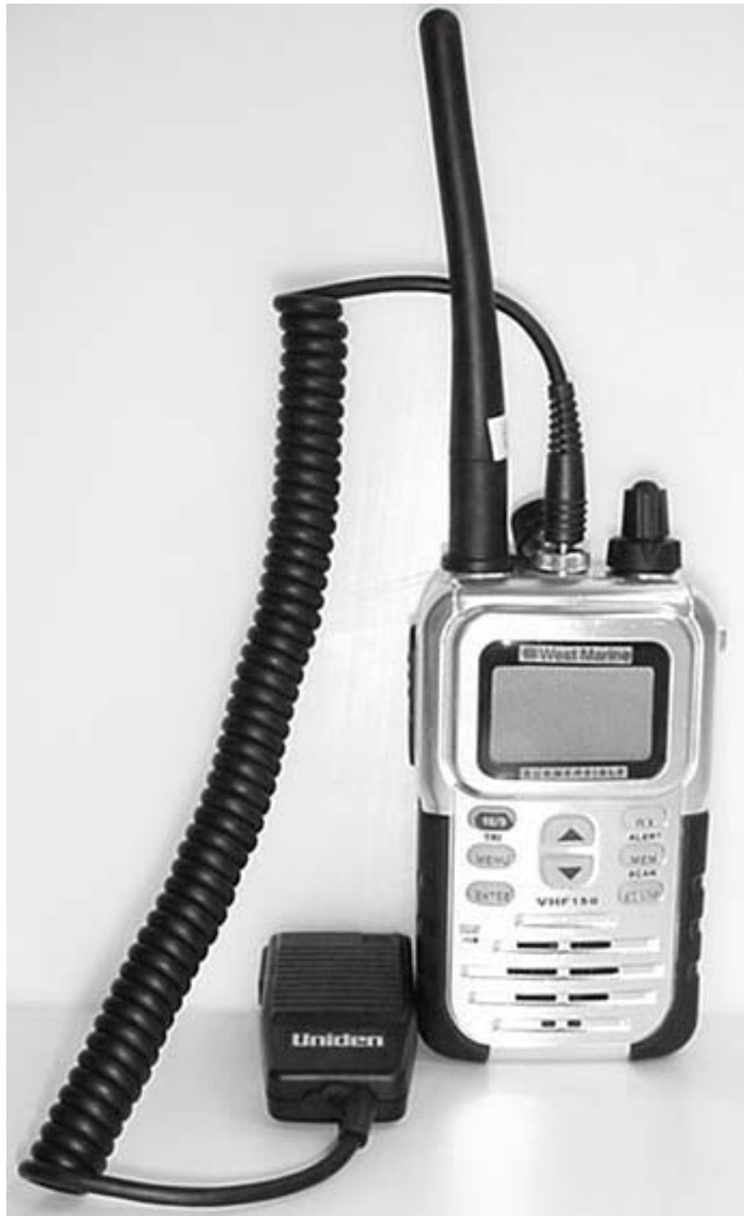
DUT with Speaker-Microphone Audio Accessory (Model: HHVTA07)
