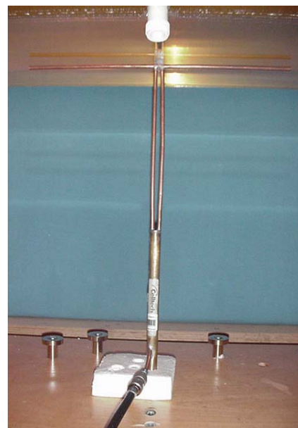
300MHz Dipole Setup
