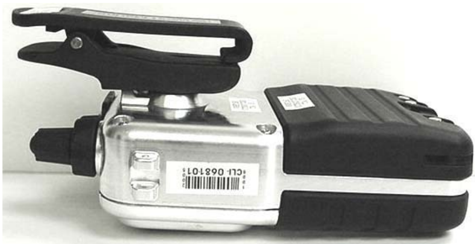
Right Side of DUT with Swivel Belt-Clip
