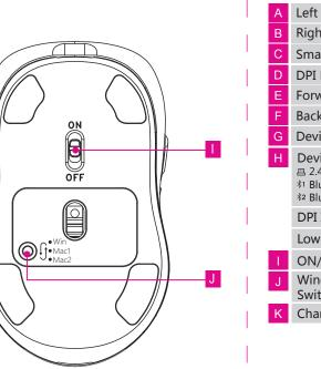
A Left Button Right Button Smart Flying Scroll Wheel \* DPI Button Forward Button Back Button Devices Switch Button Devices Indicators: □ 2.4G White Indicator ₹1 Bluetooth 1 Blue Indicator \$2 Bluetooth 2 Green Indicator **DPI** Indicator Low power indicator ON/OFF Button Windows/Mac OS Switch Button K Charging indicator light
