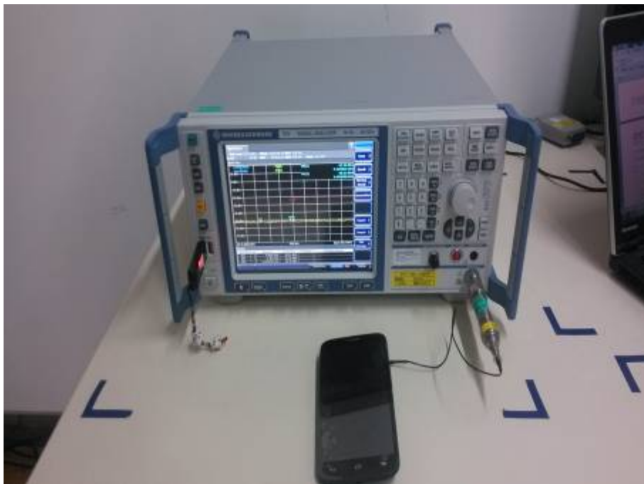
Spurious RF Conducted Emissions Test setup
