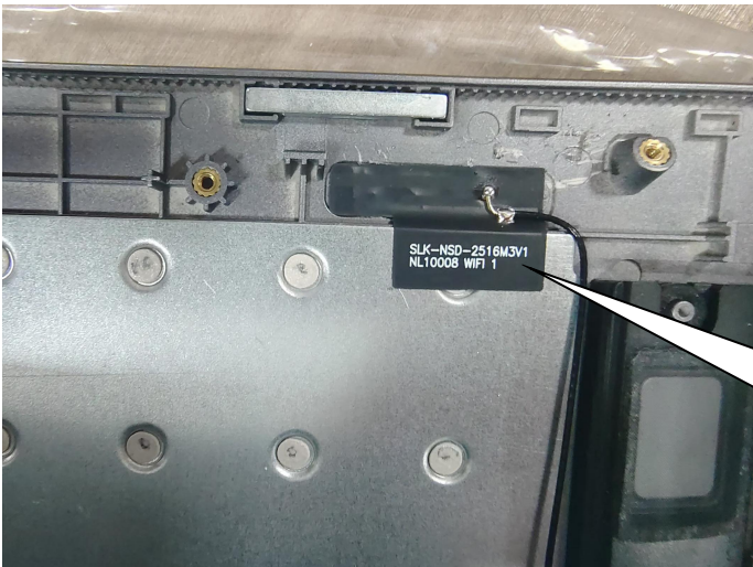
WIFI Main antenna
