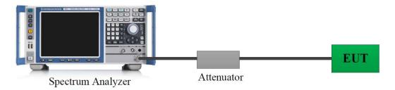
A short RF cable with low cable loss connected to the EUT antenna port, which was provided by manufacturer. The cable loss of this RF cable was offset into the setting of test equipment, which was provided by manufacturer **A**.
