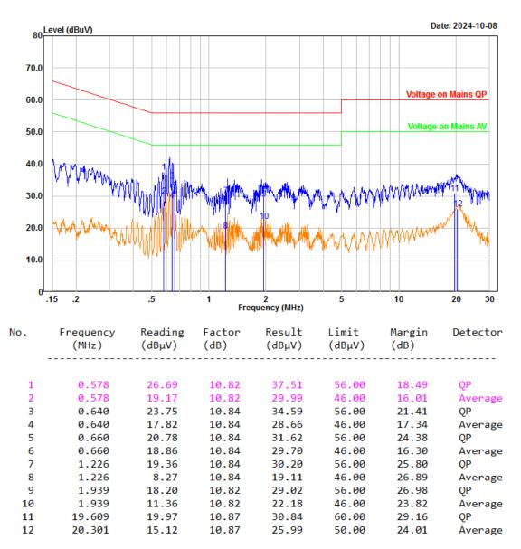
Project No.: 2402W91377E-RF Port: neutral Test Mode: Transmitting Note: BT BDR Low channel Serial No.: 2QZ4-5 Tester: Yukin Qiu
