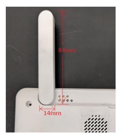
Figure 1 Physical dimension (mm)
