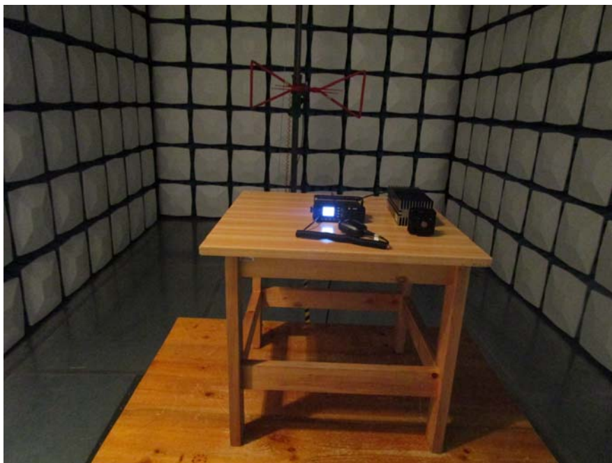
Radiated Emission View (Below 1 GHz) Vehicle Mounted
