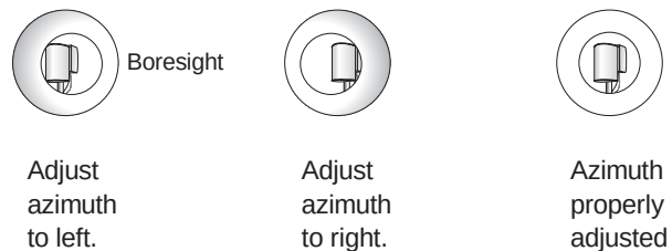
Figure 6-14 Using the boresight to adjust azimuth
