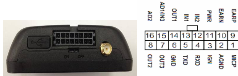
Figure 2. The 16 PIN Connector on the GV304N
