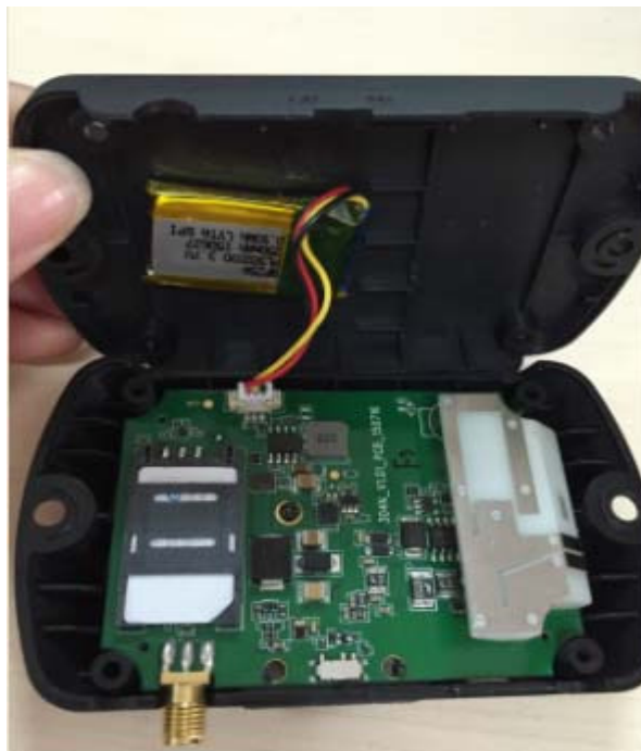
Figure 6. Backup Battery Installation
