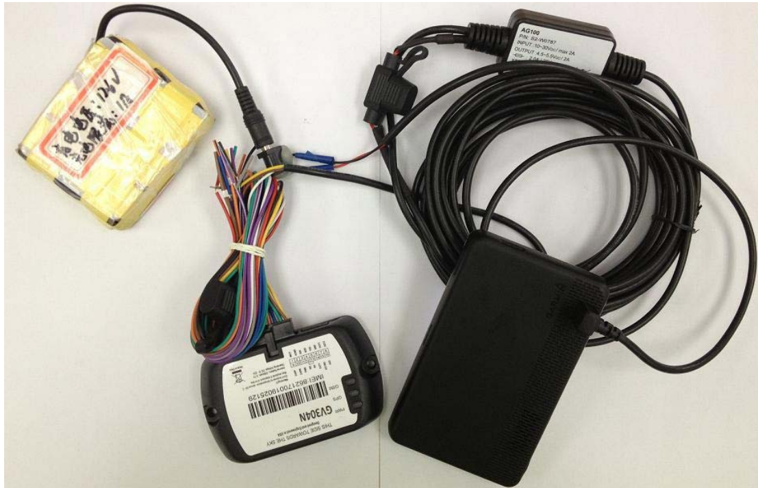
Figure 18. GV304N connection with Garmin GPS set
