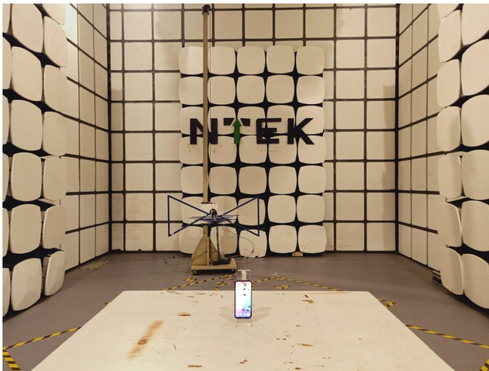
Radiated Measurement Photos(30MHz~1GHz )
