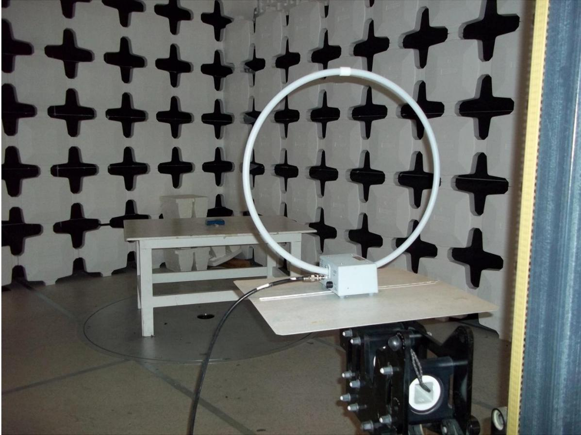
**Figure 6. Radiated Emissions Test Setup, 9 kHz - 30 MHz**
