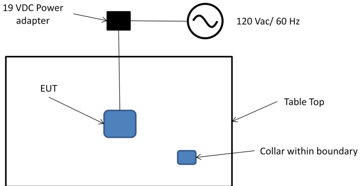
**Figure 2. Block Diagram of Test Configuration**
