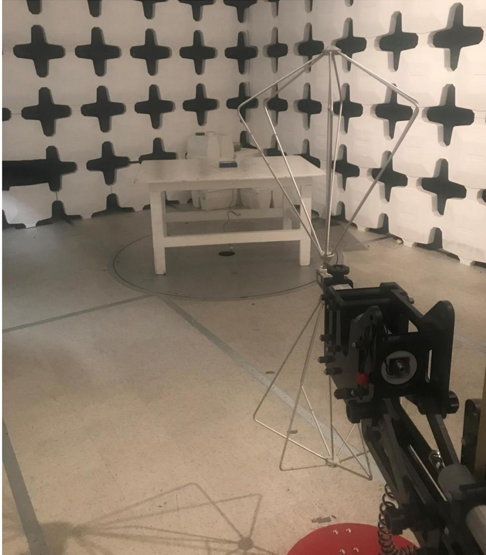
**Figure 7. Radiated Emissions Test Setup, 30 - 200 MHz**
