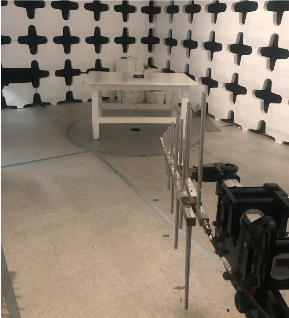
**Figure 8. Radiated Emissions Test Setup, 200 - 1000 MHz**
