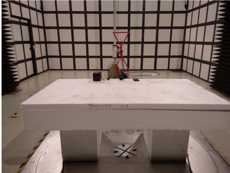
Radiated Disturbances Rear Side (Below 1GHz)
