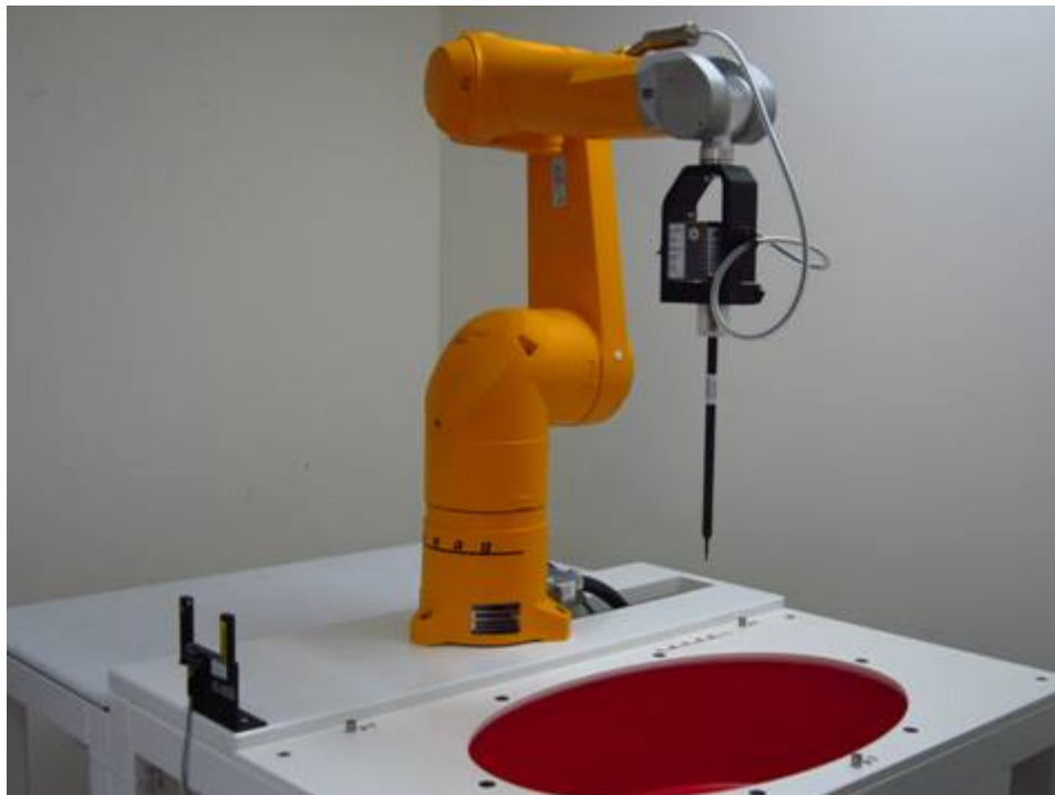
Fig.1 Photograph of the SAR measurement system
