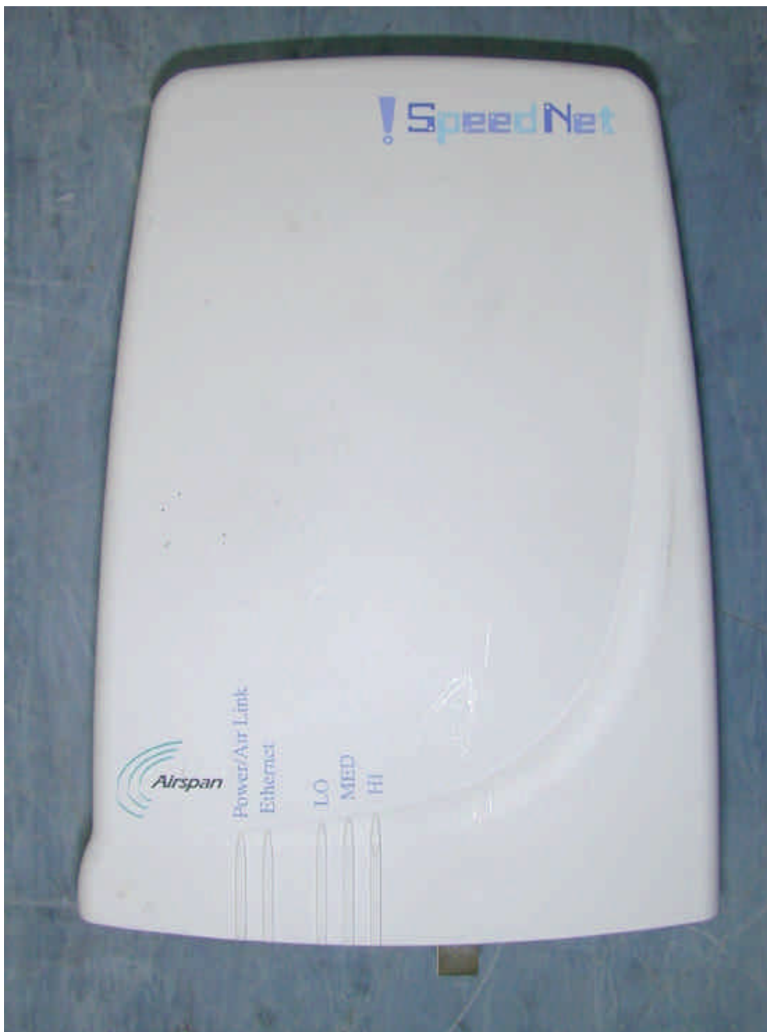
Photograph No.1 IDR 900 MHz indoor radio adapter Front view
