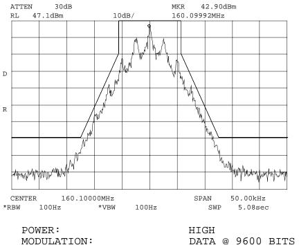
DATA @ 9600 BITS PER SECOND MASK: D, VHF/UHF 12.5kHz BW
