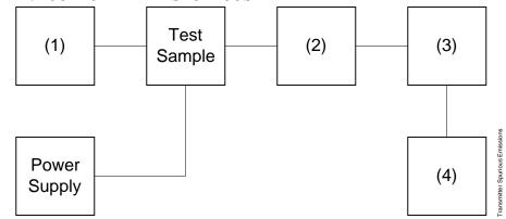
Asset Description s/n (as applicable) (1) AUDIO OSCILLATOR/GENERATOR i00010 HP 204D 1105A04683 i00017 HP 8903A 2216A01753 i00012 HP 3312A 1432A11250 (2) COAXIAL ATTENUATOR i00122 Narda 766-10 7802 i00123 Narda 766-10 7802A i00069 Bird 8329 (30 dB) 1006 i00113 Sierra 661A-3D 1059 (3) FILTERS; NOTCH, HP, LP, BP i00126 Eagle TNF-1 100-250 i00125 Eagle TNF-1 50-60 i00124 Eagle TNF-1 250-850
