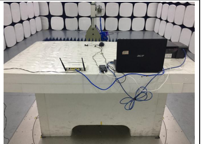
Radiated Emissions Test Setup Above 1GHz
