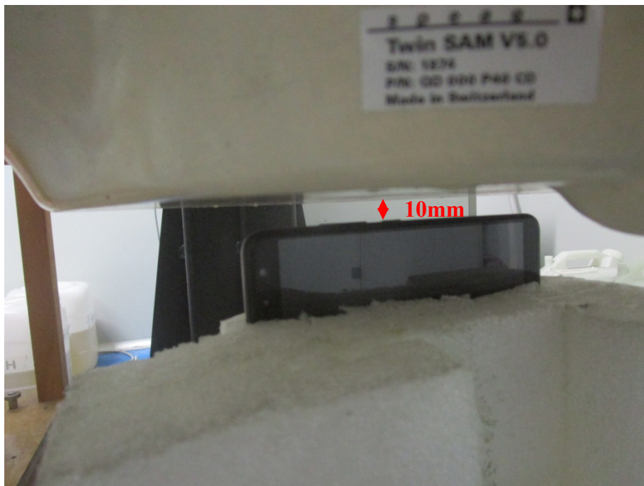
Body Left Setup Photo (10mm)
