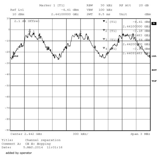
Test: 15c.8; Frequency = 2441, Mode = BT transmit using 2 Mbps with PI/4 DQPSK modulation
