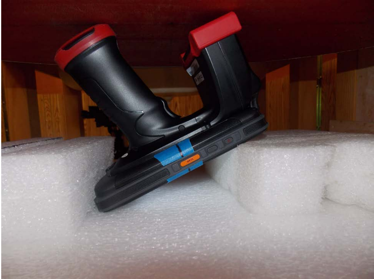
Test Position Back RFID Testing 0 mm Gap
