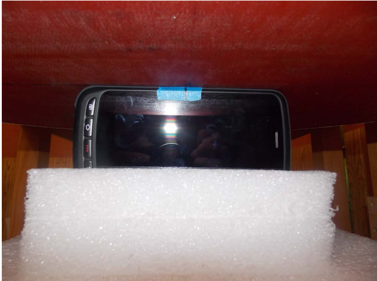
Test Position Left Testing 0 mm Gap
