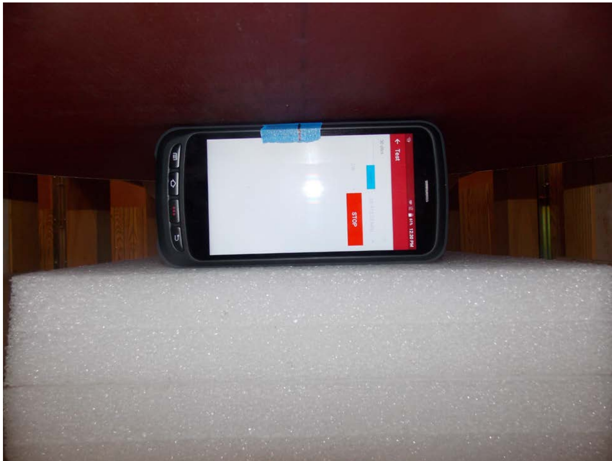
Test Position Left RFID Testing 0 mm Gap
