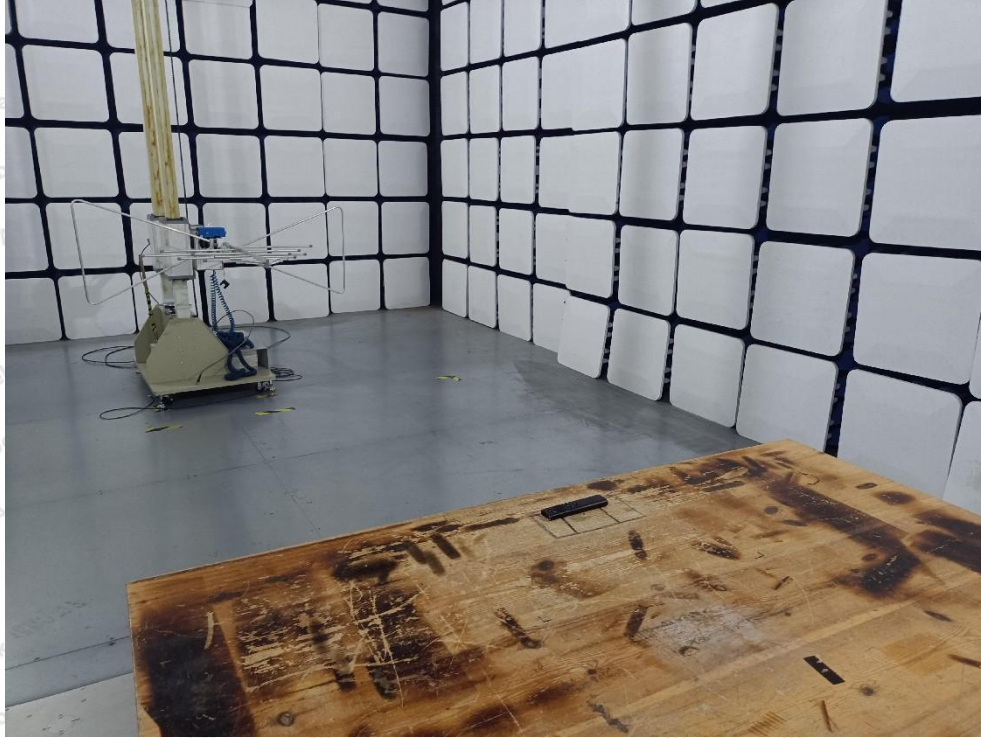
Photo of Radiation Emission Test (below 1GHz)
