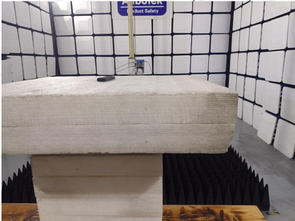
Photo of Radiation Emission Test (above 1GHz)
