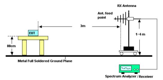
(C) Radiated Emission Test-Up Frequency Above 1GHz
