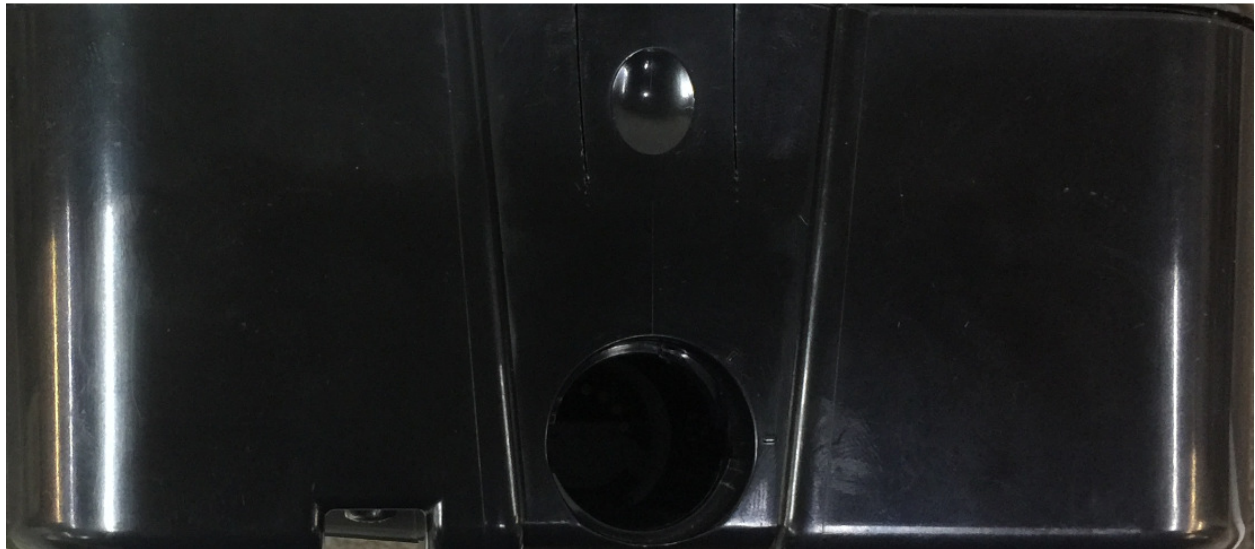
Figure 14. RAC00-16953, Battery Port and AC/DC Input Port
