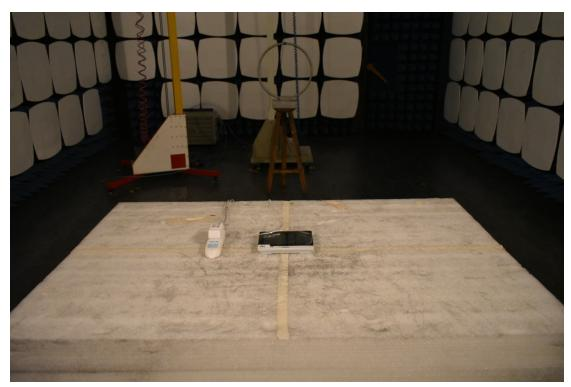
3. Radiated emission (9KHz-30MHz)
