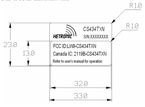
Note: Measurements in millimeters.
