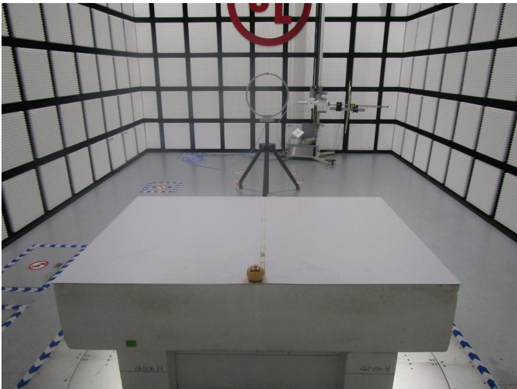
Radiated Disturbance below 30 MHz
