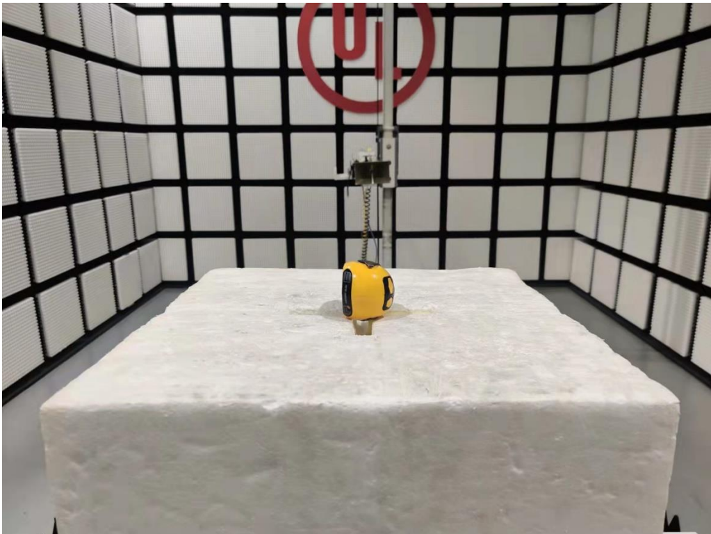
Radiated Disturbance Setup (Above 1 GHz – Y axis)
