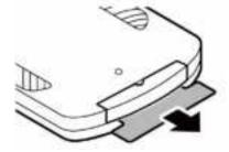
To replace a new battery, please refer to the figure shown below. When inserting a battery, be sure to do so in the proper direction.
