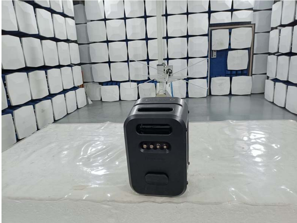
Radiated Emission Test Setup:
